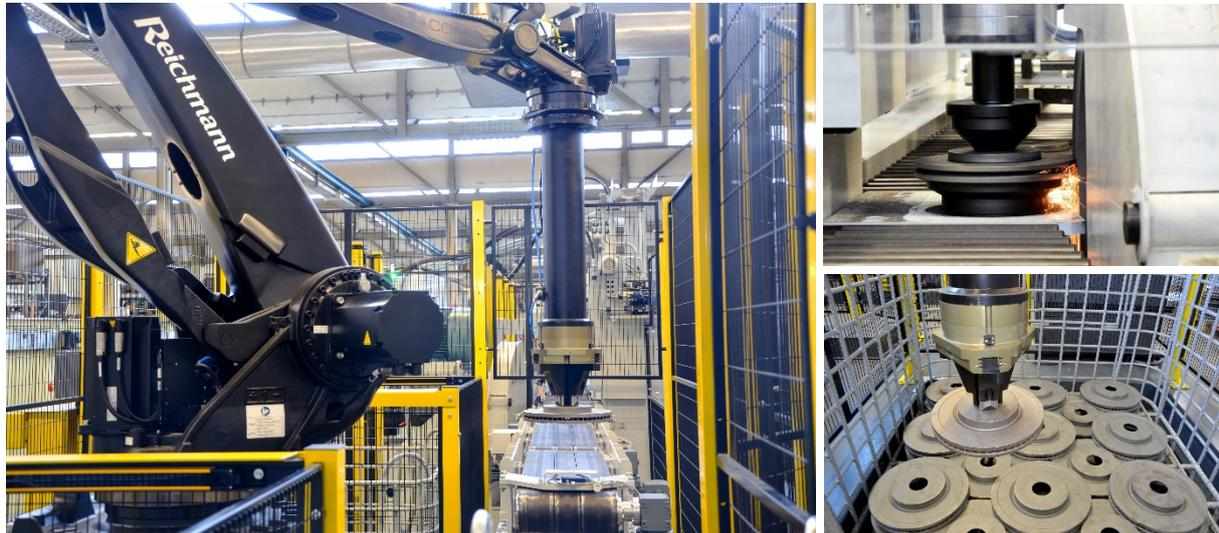
**In foundries for car and truck brake discs and drums there is a high demand for automated solutions from Reichmann Casting Finishing. For further processing of round parts in the foundry, sprue residues must be removed from the castings. Automated processes are needed here to relieve the staff, increase productivity and thus save costs and time. This year, Reichmann will be delivering 14 grinding lines for deburring round parts to customers worldwide.**
